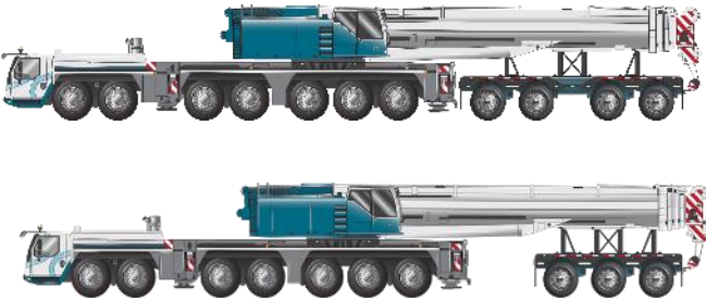
Reference vehicle 7a 6+ axle all-terrain mobile crane with reduced axle mass
