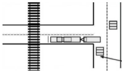
Each level crossing on the network was assessed to ensure a safe stacking for combinations of up to 30.0 metres in length.
