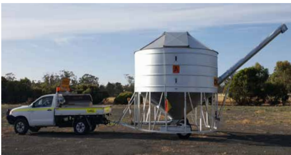
Figure 1: Field bin with an auger attachment towed by a light vehicle
