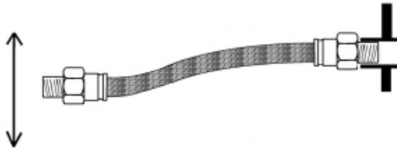
Because braided line is more rigid, it does not always pass this test. This might be fine for drag and track racing conditions where suspension movements are limited and the components are regularly checked and often replaced, particularly if the vehicle is involved in a crash. But it is not so good for road use where the brake hoses may not be inspected for many years.
