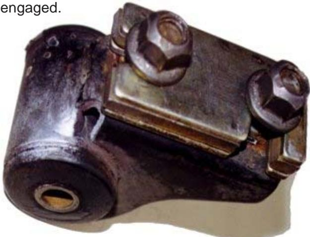
This is particularly dangerous as, apart from the risk of the thread stripping, the nuts are required to be self-locking (either “crimped thread” as in the example shown or “NyLock” type as supplied by Ford with the long stud version of the bush). Self locking nuts require the studs to project right through if they are going to work and ensure they do not loosen in service.
