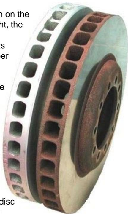
As if this is not bad enough, in this case, the centre mounting plate has also separated from the rotor and can be freely rotated inside the cast rotor. The cast rotor is normally fixed to the centre steel mounting plate by crimping the steel plate over extensions to the rotor vanes as can be seen in the photo below.
