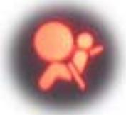
Ah Ha! The diagnostic system is smarter than that. Every time the engine is started the indicator lamp first comes on to show that the globe is OK and the system is being checked and it then goes off if everything is correct. So it's simple to check that the airbag is present and functional. Turn the ignition on or start the engine and watch the indicator light.
