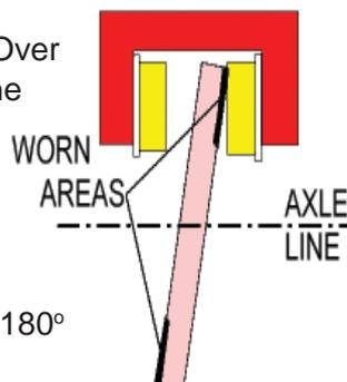
These two areas only need to be worn by 10 to 20 microns for brake shuddering to occur. When you consider the way the rotor has been worn and that there are 27 microns to one thousandth of an inch, you can see that running a dial gauge over the rotor will not detect DTV. In fact, the dial gauge will show even less runout than before the wear occurred. You will need to use a micrometer to measure the thickness at about eight places around the rotor to detect DTV.
