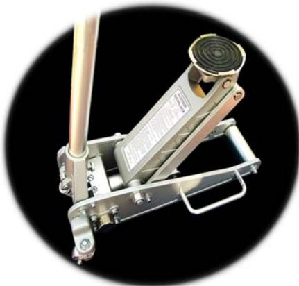
How many of you have an old trolley jack that slowly creeps down? Why does it creep down? Because an oil seal has deteriorated and sooner or later [hopefully later] that seal is going to let go suddenly and completely. You may not
