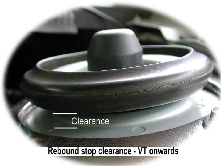
If the bush is badly worn or deteriorated the top of the strut shaft will project further through the strut tower taking the rebound stop with it and the clearance between the “rubber tyre” and the top of the strut tower will be greater than normal. This will also result a greater than normal movement of the rebound stop between the on-ground and raised conditions.
