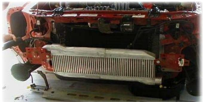
However modifying the front structure of the vehicle as above to fit that larger unit will definitely affect the compliance of the vehicle as well as making it potentially unsafe and this will attract a defect notice.
