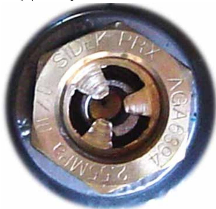
All such valves as shown in the picture above need to be replaced as a matter of urgency. If any LPG fuelled vehicle with one of these valves is presented to you for a roadworthy you should not issue a RWC until the valve has been replaced.
