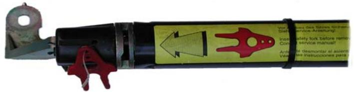
Then the seats are re-fitted still with the deployed pretensioners and to hide the problem the warning tags are cut off.
