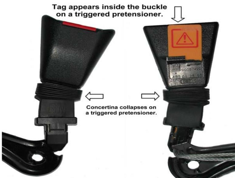
Some of these mechanical seatbelt buckle pretensioners can be inadvertently triggered if the proper removal and replacement procedures are not followed.
