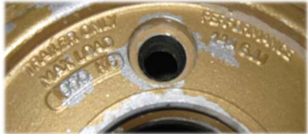
One of the requirements of AS 1638 is impact testing to simulate kerb impacts and as can be seen from the picture below, these wheels seem to be very brittle. What appears to have been a relatively light impact to the lip of the rim has caused a very significant failure to the body of the rim.
