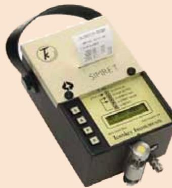
Turnkey Instruments Brake Decelerometer
