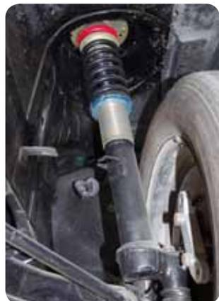
Fitting coil-overs and alternative struts presents some additional issues in making sure that the spring tension is set up correctly. Having unbalanced tensions can have unfortunate effects on the vehicle's stability. A road test checking for balanced handling over bumps and also while cornering and braking is mandatory.
