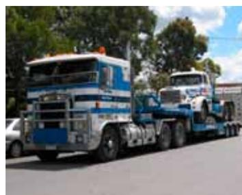
**Low deck semi-trailer** – is a prime mover and semi-trailer combination where the semi-trailer has a low deck and loading ramps or a tilt deck for winching a disabled vehicle on to its deck.
