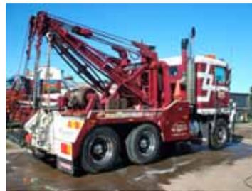
**Hook tow truck** – has a cable and hook mechanism to lift and tow vehicles.
