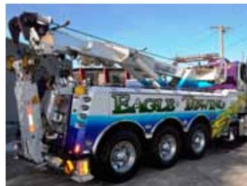
**Underlift tow truck** – has a rigid arm that extends under disabled vehicles and lifts them off the road surface for towing.
