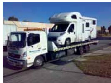
**Tilt deck truck** – is a rigid truck where the deck can hydraulically tilt to enable a disabled vehicle to be winched on to its back.
