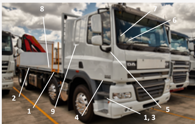
Figure 6.3 Primary structure components
