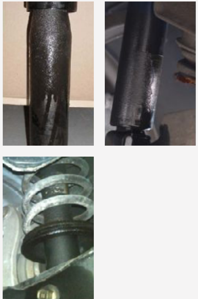
Figure 4.5 Examples of leaking shock absorbers
