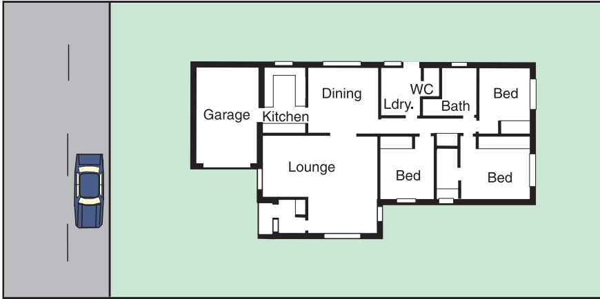
A suggested house layout with arterial road at front. Bedrooms are to the rear of the house with garage forming sound barrier.
