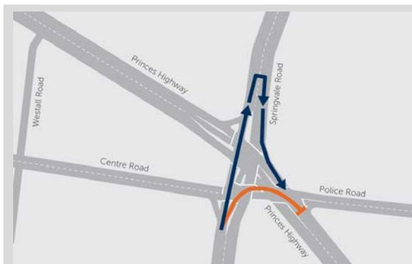
Figure 5 Redirecting a right turn using a "U" turn
