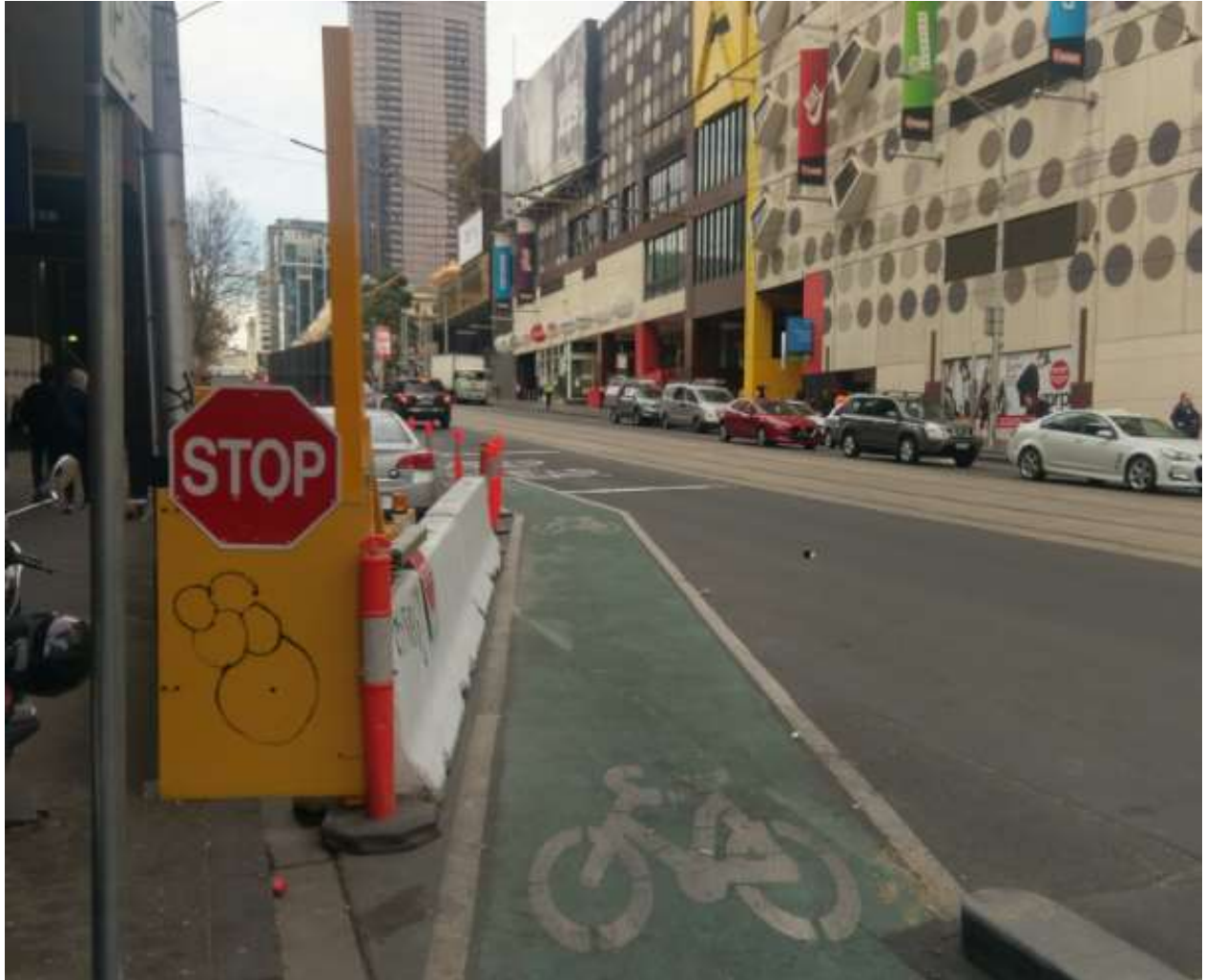
FIGURE 19: REMOTE CONTROLLED BARRIER THAT DROPS TO HORIZONTAL FOR THE CONTROL AND COORDINATION OF CYCLISTS
