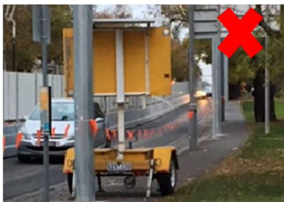
FIGURE 15: FOOTPATH BLOCKED BY VMS SIGN
