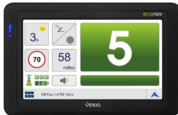
**Figure 1** The visual display of the ‘Econav’ system showing, for example, information on ideal gear (top right) acceleration and speed
