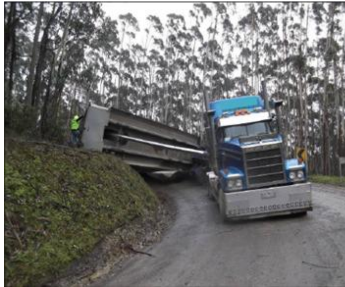
The potential to fall onto adjacent traffic lanes, people, plant and vehicles
