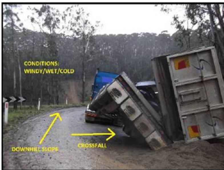
Semi tipper overturns with slight downhill gradient and cross fall
