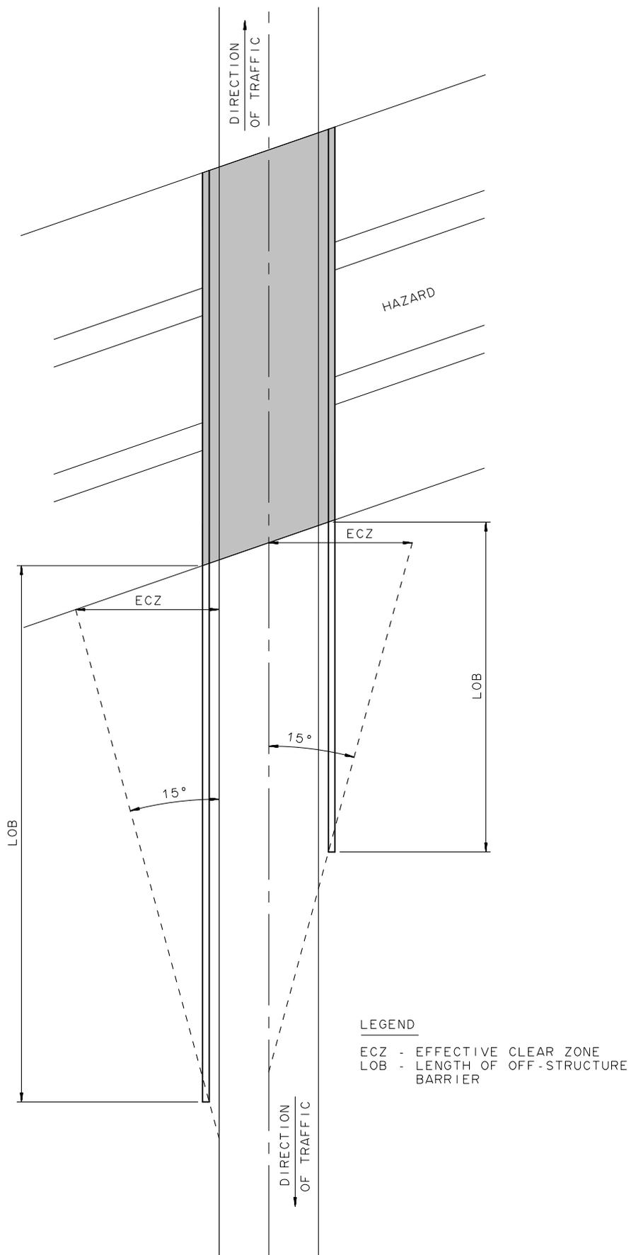
**Figure B2 - Geometry of a Skew Bridge**
