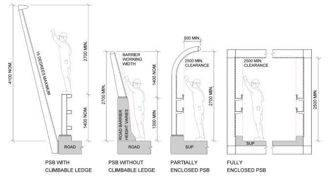
Figure 1 – Examples of Typical Public Safety Barriers showing minimum height and orientation requirements
