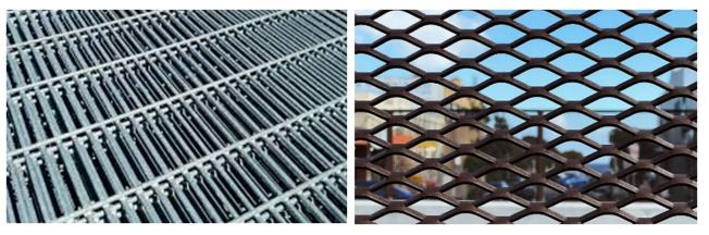
Figure 12 - Welded mesh
