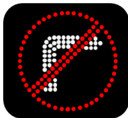
Figure 4.2 - Sign partially off during flash cycle
