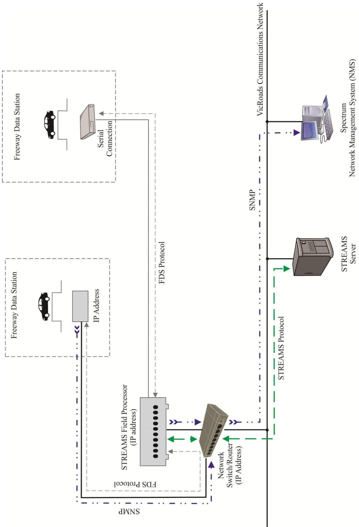
**Figure A1 - LUS connected to STREAMS**
