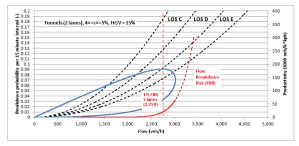
Figure 2-6: Breakdown probability and productivity plotted against flow rate (2 lane tunnels)
