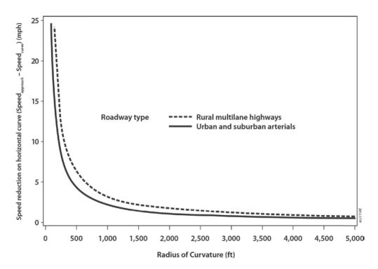
Figure 3-11: Speed reduction on curves (Harwood et al., 2014)
