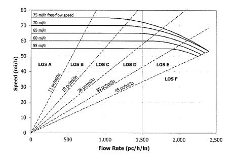
Figure 1-1: General relationship between speed and flow rate (Source: HCM 2016)
