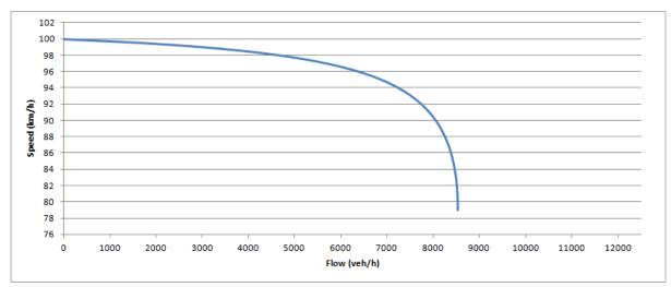
Figure 2-17: Average vehicle speed for 5 lane cross-sections (100 km/h speed limit)
