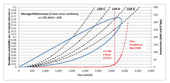
Figure 2-1: Breakdown probability and productivity plotted against flow rate (2 lane cross-sections)
