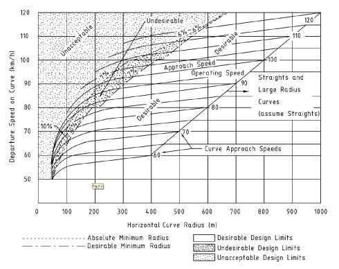
Figure 3-10: Car deceleration on curves (Austroads, 2016)
