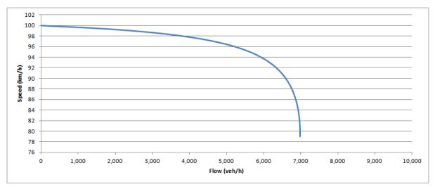
Figure 2-16: Average vehicle speed for 4 lane cross-sections (100 km/h speed limit)
