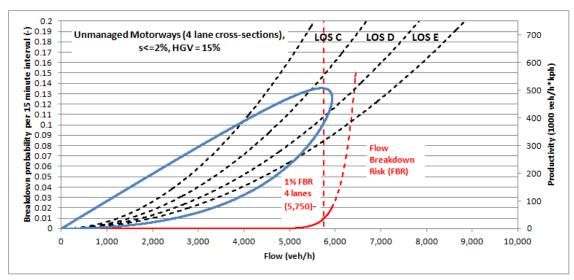
Figure 2-12: Breakdown probability and productivity plotted against flow rate (4 lane cross-sections)
