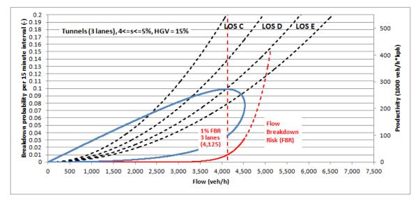
Figure 2-7: Breakdown probability and productivity plotted against flow rate (3 lane tunnels)
