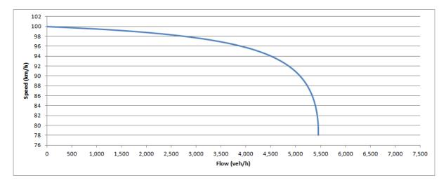
Figure 2-15: Average vehicle speed for 3 lane cross-sections (100 km/h speed limit)
