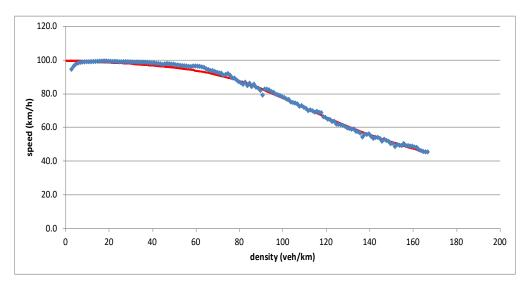
Figure 3-3: Speed-density relation for cross-section 14587IB (Monash Freeway - Jacksons to Wellington Road, inbound, 4 lanes) - measured values (1 hour rolling averages aggregated for density classes) and van Aerde curve approximation (elimination of downstream bottleneck influence – hence no very high densities)
