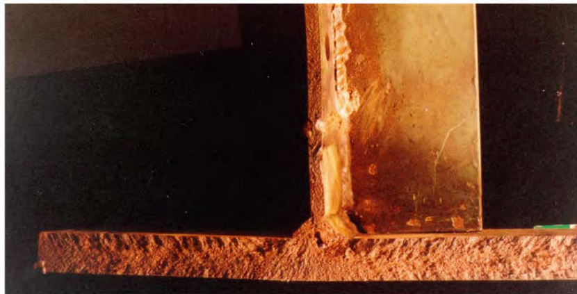
Figure 45: Typical fatigue crack across a repaired flange butt weld (FHWA-IF-13-020)
