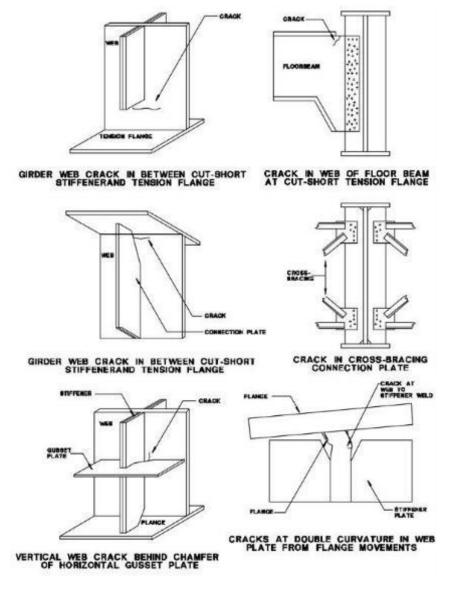
Figure 1.1.3.3 (a) Common locations susceptible to cracking
