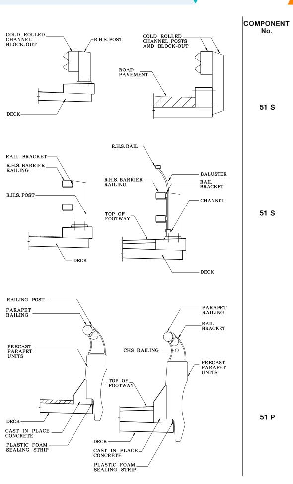
FIG. 15 - BRIDGE RAILING / BARRIER
