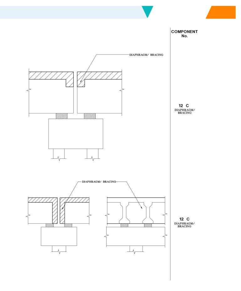
FIG. 8.2 - LOAD BEARING DIAPHRAGMS & DIAPHRAGM/ BRACING (Sheet 2 of 2)
