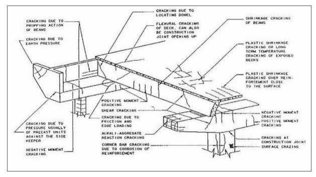
Figure 1.1.2.7 (a) Types and location of cracks in concrete structures
