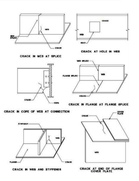
Figure 1.1.3.3 (b) Common locations susceptible to cracking
