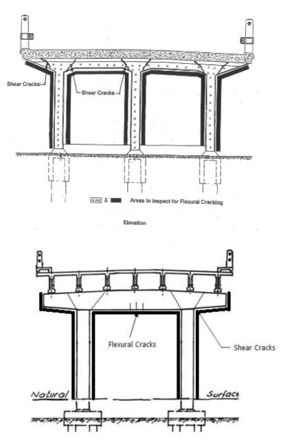
Figure 1.17 Bridge substructure inspection areas
