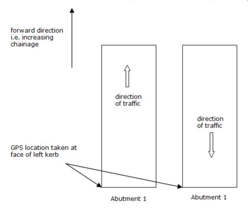
Figure 3.6.5.1.4 GPS location for a dual carriageway
