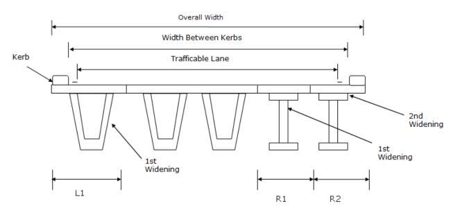
Figure 3.6.5.1.2 Bridge widths (superstructure only)
