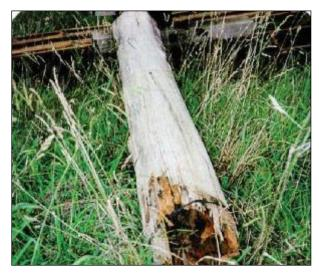
Figure 1.1.4.1 Pile failure resulting from heartwood rot.
