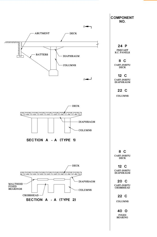
FIG. 7 - CAST - INSITU FLAT SLAB BRIDGES
