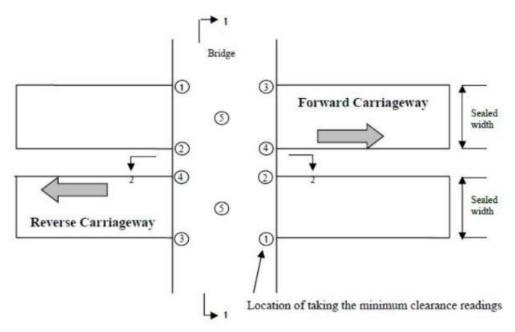
Figure 3.6.4 – Location of taking the minimum clearance readings
