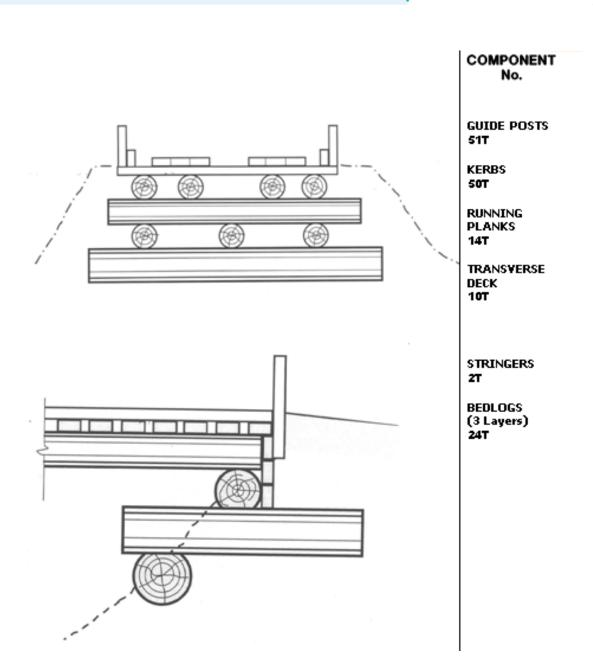
FIG. 10.1A - VICFOREST TYPE TIMBER BRIDGE ABUTMENT
