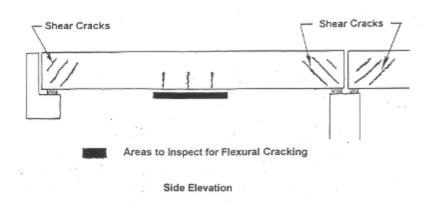
Figure 1.1.1 U-Slab side elevation
