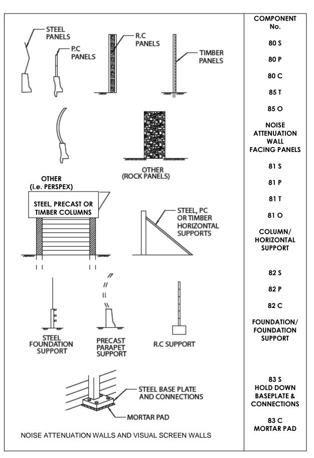
FIG 23 - NOISE ATTENUATION WALLS AND VISUAL SCREEN WALLS
