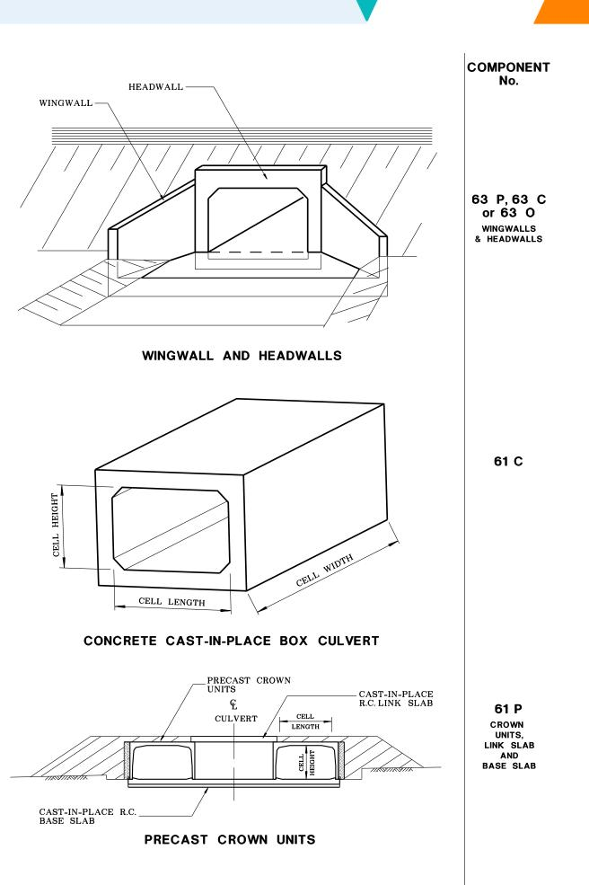
FIG. 16.2 - CULVERTS (Sheet 2 of 2)
