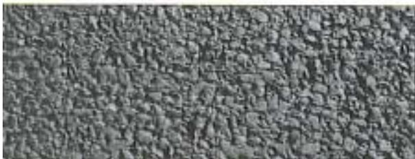
*Structure and appearance of Open Graded Asphalt*
