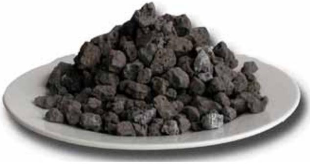
Figure 1 – Steel Furnace Slag Aggregate <sup>2</sup>
