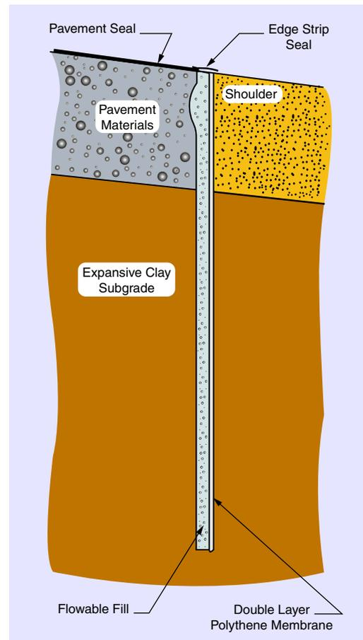
**Figure 1. Cross-section of Barrier**
