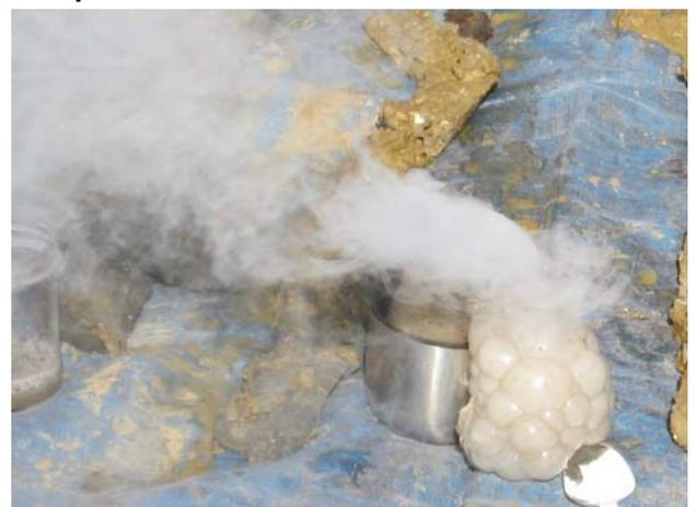
**Figure 6: Using hot water to accelerate oxidation of soil with hydrogen peroxide solution.**
