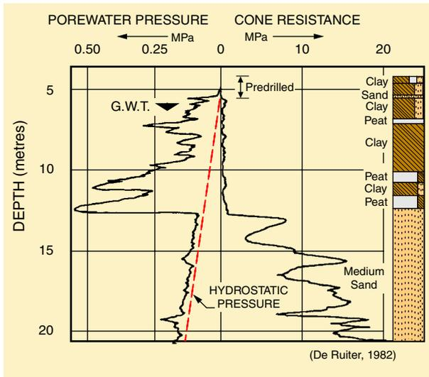
**Figure 2: Typical Fugro Piezo-Cone Penetrometer Test Result**
