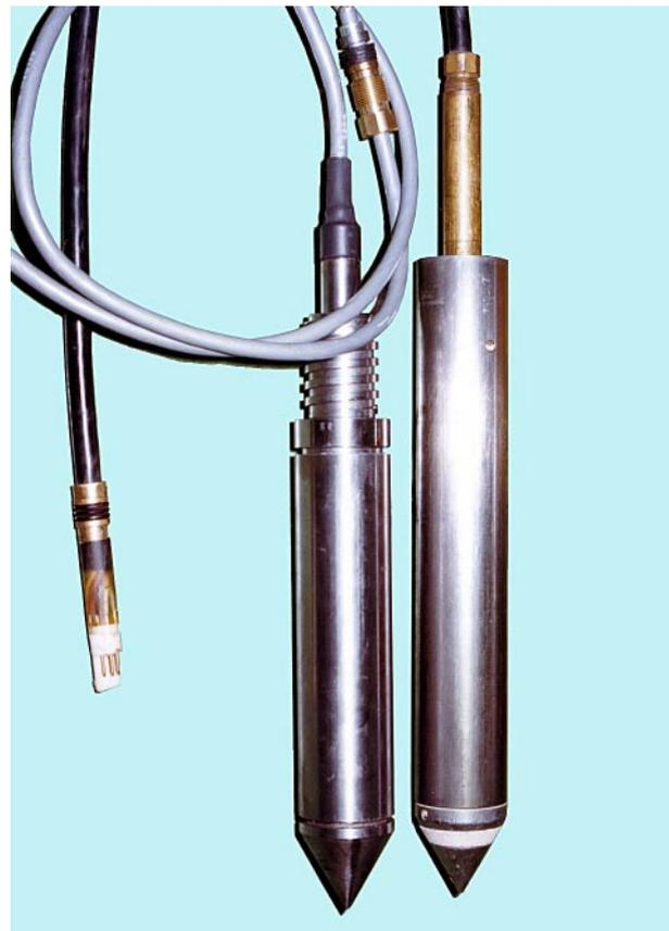
**Figure 1: Fugro Piezo-Cone Penetrometer (Right) with standard Friction Cone Penetrometer (Left)**
