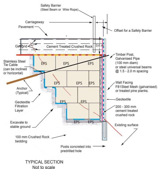
Figure 1: Typical Crosssection of EPS Repair
