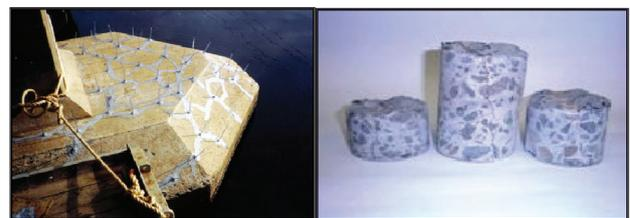
Fig. 3. Crack Injection with Epoxy Resin for significant ASR Repairs (L), Verification of depth of penetration of epoxy injection
