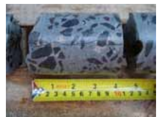
Fig 8 - Cores showing epoxy penetration
