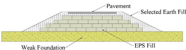
Figure 1. Typical EPS Fill Embankment Cross-section
