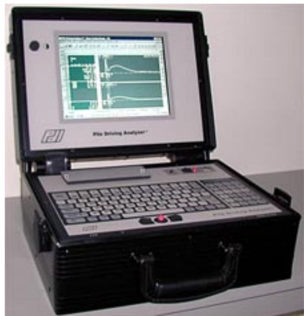
**Figure 2. Pile Driving Analyzer**
