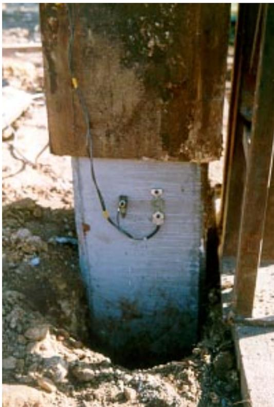
**Figure 1. Pile with Strain Gauge and Accelerometer**
