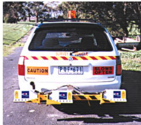
**Figure 1. Laser Profiler**
