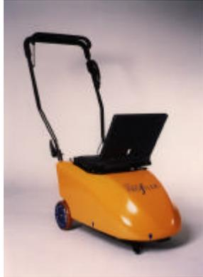
**Figure 2. ARRB TR Walking Profiler**
