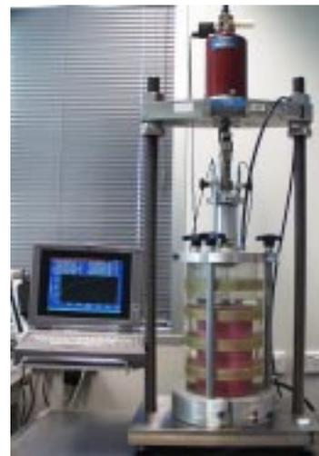
**Figure 1 Repeated Load Triaxial Test Equipment**
