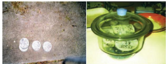
Figure 1 – Standard test cylinder cut into four slices. Following oven drying, specimens are allowed to cool in a desiccator
