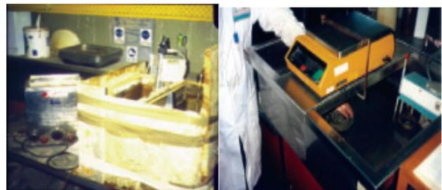
Figure 2 – Specimens are immersed in water at standard temperature followed by boiling as part of the process. Specimens are then weighed under water
