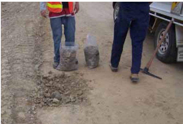
Figure 12 Examples of poor sampling practice. Both photos show sampling not to full layer depth, sides of hole not vertical, significant material (including oversize) not taken in sample
