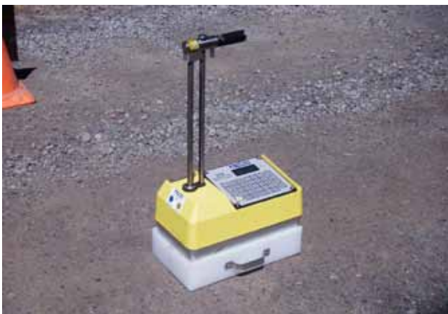
Figure 1 NDG Soil Meter – Setup for standard counts, seated on reference block. Note position of block handle to keypad. Gauge handle at top of index rod.
