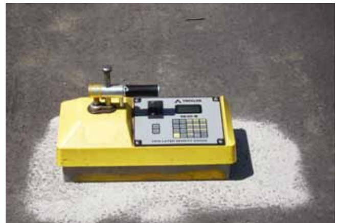
Figure 13 NDG thin-layer asphalt gauge in test mode on an asphalt surface (fine sand spread at minimum thickness)
