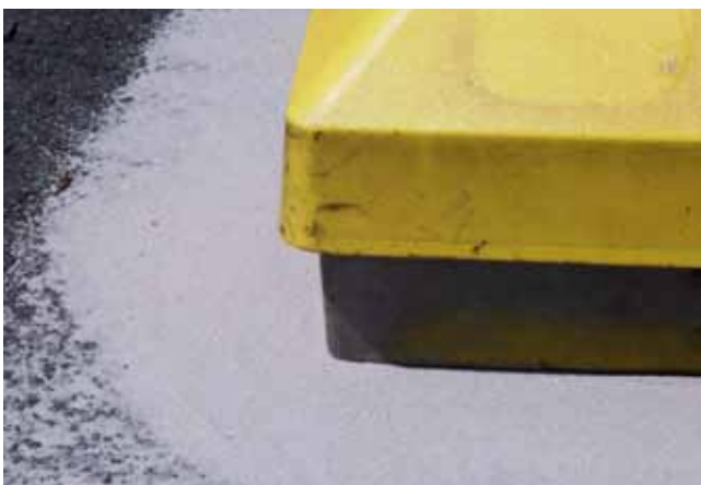
Figure 10 Fine sand forming an added layer – not to method
