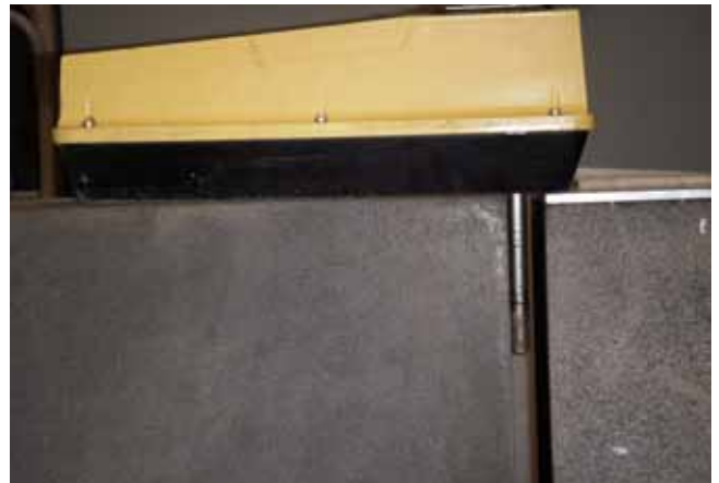
Figure 7 Cross section of NDG showing test probe against detector side of access hole
