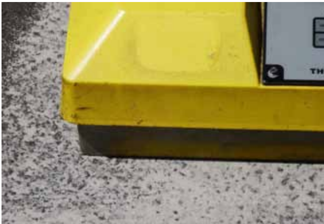
Figure 9 Fine sand at minimum thickness – not an added layer
