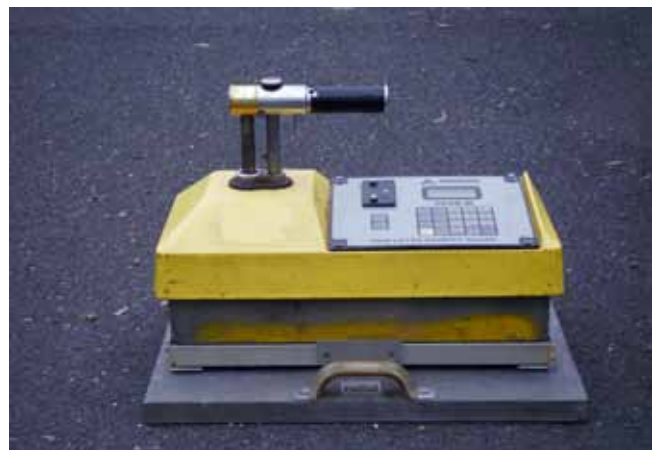
Figure 2 NDG Asphalt thin-layer gauge – Setup for standard counts. Note position of reference plate handle to keypad. Gauge handle at top of index rod.
