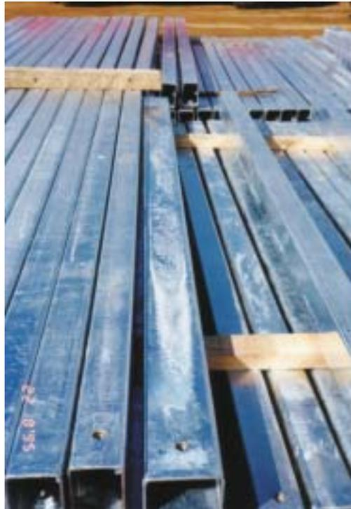
**Figure 8.1:** *The storage of galvanized components should allow for air circulation, to avoid wet storage stain and formation of white zinc corrosion product.*
