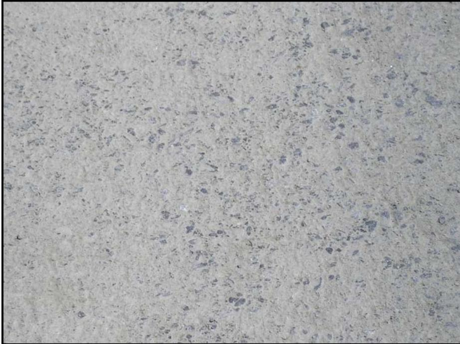
**Figure 4 : Well Prepared Surface - Uniform Texture**
