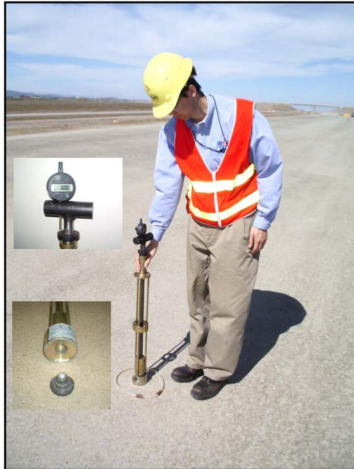
**Figure 10 : Ball Embedment Penetrometer**
