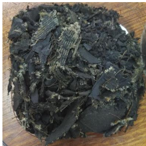
Figure 3.3: Shredded passenger vehicle tyre (contains nylon)
