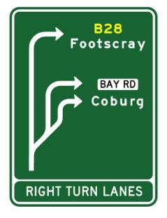
In this example, access to a further turnoff is from the right most exclusive left turn lane. In this example, additional right turn lanes for an intermediate intersection develop from an exclusive right turn lane for a downstream intersection.
