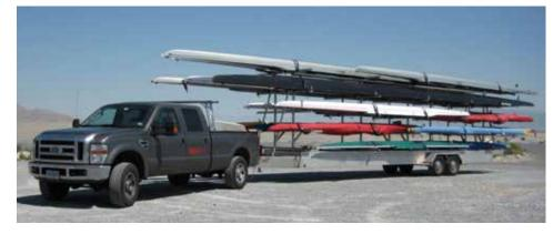
Figure 2: Example of a trailer combination transporting rowing shells
