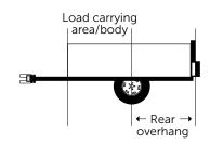
Limiting a vehicle's rear overhang ensures that when turning at an intersection or a roundabout the rear of the vehicle will stay within its lane and not impede other road users.
