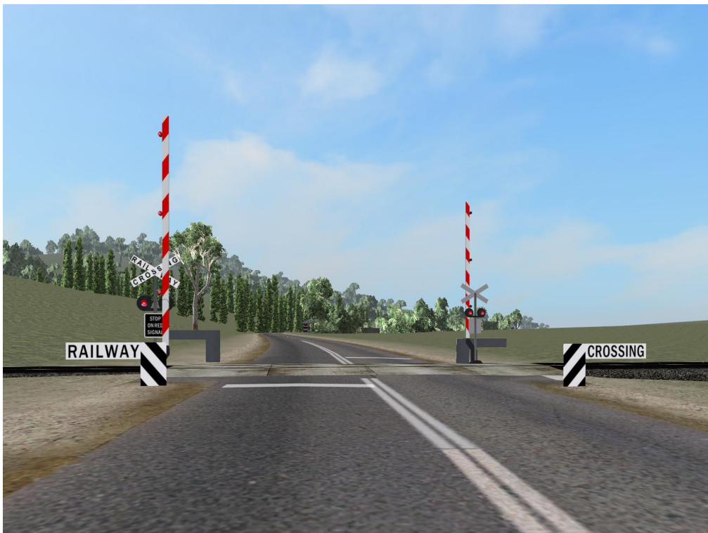
Figure 6c. Screen shot of approach to level crossing with red flashing light controls PLUS boom barrier ('Boom'). Barriers raised.
