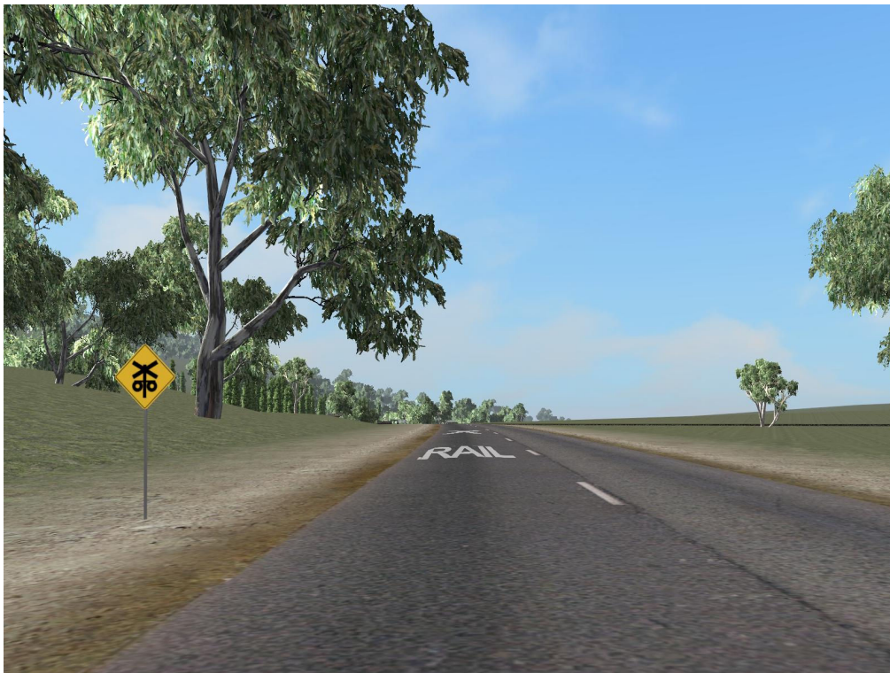
Figure 4b. Screen image of approach to level crossing with standard Australian red flashing light controls ('FlashL').
