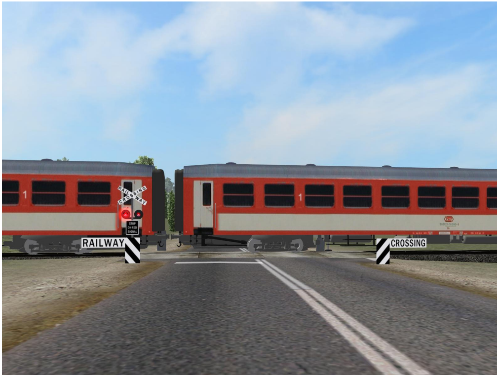
Figure 4c. Screen image of level crossing with standard Australian red flashing light controls ('FlashL').
